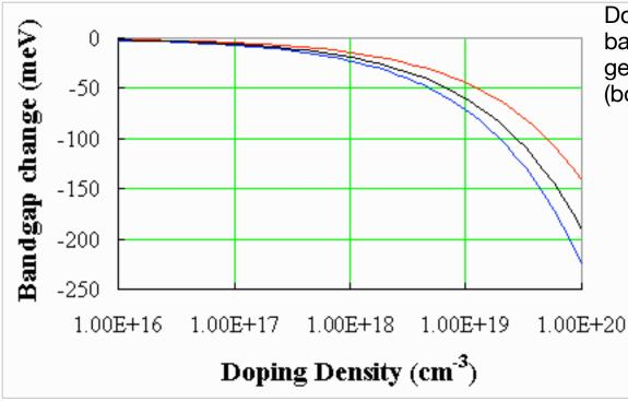
Doping dependence of the energy bandgap of GaAs (top/red curve), germanium (black curve) and silicon (bottom/blue curve).
