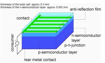
The electrons move from the p-type to the n type while the holes move in the reverse direction. If they reach the boundaries than we have a current: electricity.
